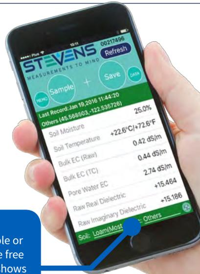
Sample data from your wirelessly connected Apple or Android smartphone. The free HydraMon app logs and shows measurements instantly and will export it as a .CSV file.
