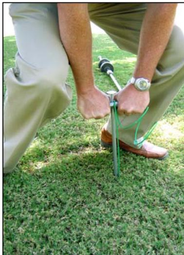
Use tee handle to "seat" sensor in bottom of hole, maximum depth is 30" (76 cm).
