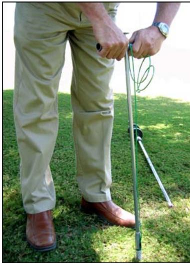
Sensor is placed on end of #1017 Insertion Tool.
