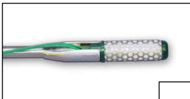
Insertion Tool with WATERMARK sensor attached.
