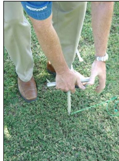
Disengage tool from sensor with ejector button.
